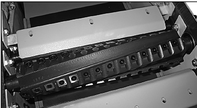
FOUR SIDED SPIRAL CUTTER BLOCK WITH HSS INSERTS
